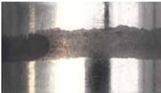
Photomicrograph of the hydraulic strut sample after chrome plating removal with PurePulse waterjet technology. (scaled at 1 in.)
