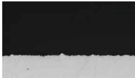
Micro image showing surface condition of the hydraulic strut sample. (200x)
